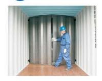
Form a V with the two panels the press into place.
