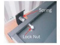
Slide spring on the shaft of the stabilizer. Push the shaft thru the hole of the panel. Secure lock nut. Make sure you see 2 to 3 full threads.
