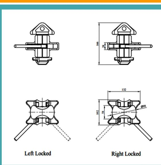
Twistlock Stacking Pins are designed for stacking shipping containers on top of each other. The containers stacking pin/cone features a plate with a locating pin on either end that slots into the holes cut out on the corner casts. The locking stacking pin/cones we provide come with a handle which can be engaged or disengaged to lock or unlock two shipping containers.
